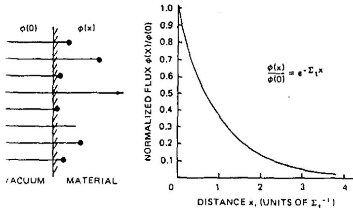
FIGURE 2-14 Exponential attenuation of a neutron beam in a material with total macroscopic cross section  $\Sigma_t$ .
